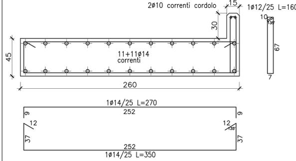
SCHEMA ARMATURA PALI Scala 1:20
